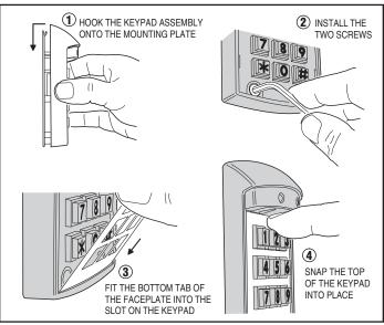
Figure 5. Connecting the Keypad to the Mounting Plate
